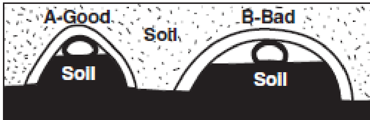
Figure 4. Rounded rake tile, A, provides snug fit for good insulation. Compare to B, which allows easy entry of hot air and breezes that dehydrate.
